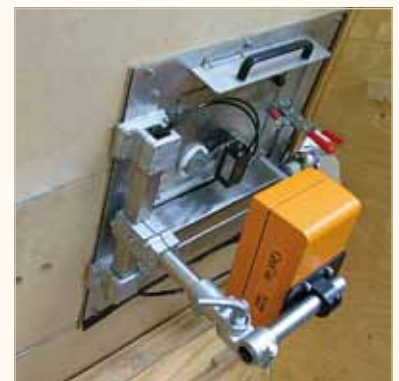
FMV in drop chute underneath dryer cyclone
